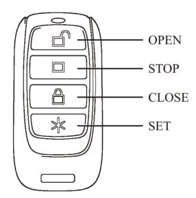
Important: There is only a "learn" button on the door opener control board. Before setting on the Transmitter, it must be coded.
