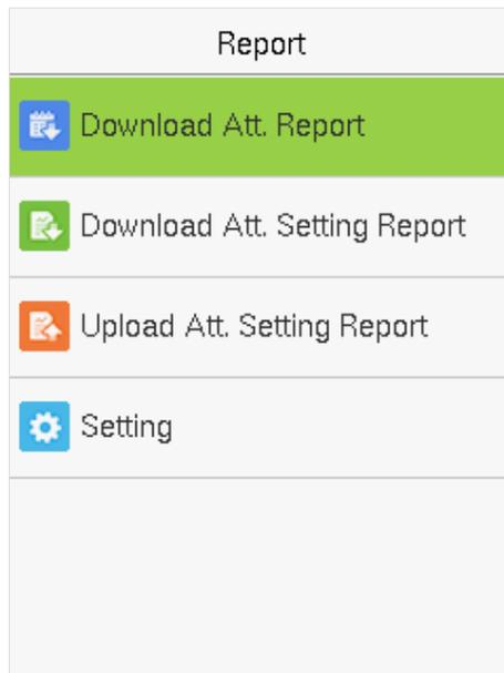
**Note:** First insert the USB flash drive into the USB slot of the machine, and then enter the main menu to perform the related operations of the **Report**.
