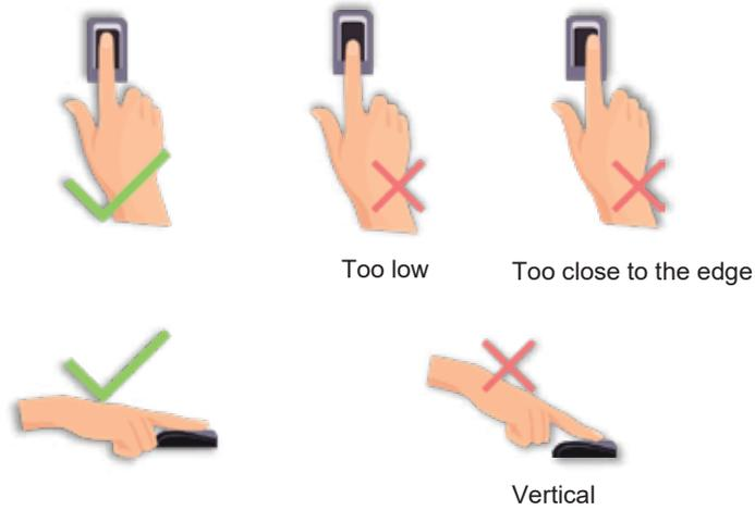
**Note:** the recommended method when pressing your fingers onto the fingerprint reader for registration and identification. Our company will assume no liability for recognition issues that may result from incorrect usage of the product. We reserve the right of final interpretation and modification concerning this point.
