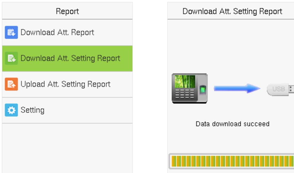
Open the setting "AttSettingE.xls" in the USB disk or SD card on a PC. Set the Shift in the Attendance setting report. The shifts that have been set on the attendance machine shall be displayed. (For more details, see [Shift Setting](#). You can modify the 24 shifts and add more shifts. After modification, the shifts shall prevail on the attendance machine.
