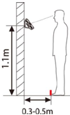
It is recommended to have a 0.3-0.5m space between the device and the customer whose height is 1.55m to 1.85m. Users may slightly move forwards and backward to improve the quality of facial images captured.
