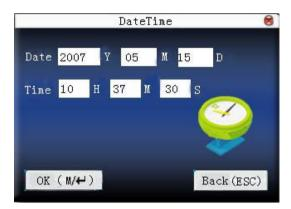
Press  $\blacktriangle/\blacktriangledown$  to move cursor to the input box. Press numeric key on small keyboard to input the value. After setting, press **menu** directly to save the setting and return to the last interface. Press "**ESC**" to cancel setting and return to the last interface.
