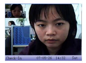
Step 3: When device prompts "Thank you", (if user has enrolled photo, the photo will be displayed.), the verification is complete.
