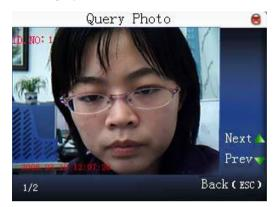
Press  $\blacktriangle/\blacktriangledown$  to search attendance photo saved in the device. The information that how many photos there are and which one is the current photo will be displayed under the photo. The taking date and time will be displayed as well.
