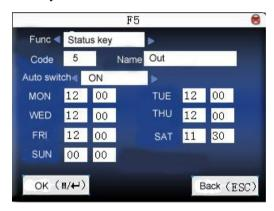
Press  $\blacktriangle/\blacktriangledown$  to move cursor to the input box. Press numeric key on small keyboard to input the value. After setting, press **menu** directly to save the setting and return to the last interface. Press "**ESC**" to cancel setting and return to the last interface.
