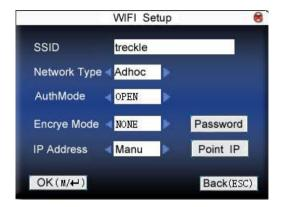
Press  $\blacktriangle/\blacktriangledown$  to switch cursor to the input box or button. Use T9 input to input network ID, which must be input, or the cursor cannot be moved to other input box. Then press  $\blacktriangledown/\blacktriangleright$  to select the item to be set or press **OK** to do corresponding operation.
