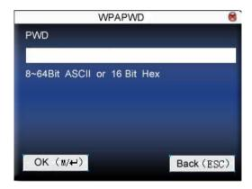
Input correct password ,set password, press **OK** or **menu** to save the setting, and then return to **wireless option** interface.
