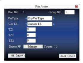
Press ▲/▼ to move cursor to the item to be set. If it is the input box, press numeric keys on small keyboard to input the value. If it is the roll box, press ৺► to switch the values. When the cursor is on "manage duress fingerprint", press ← to enter duress fingerprint management. After setting, press ← or menu directly to return to the last interface. Press "ESC" to cancel setting and return to the last interface.
