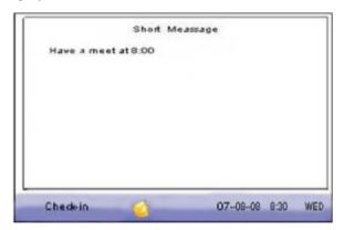
The information display time length is 30 seconds. During this period, user verification can be done. Close the current display to enter verification interface.
