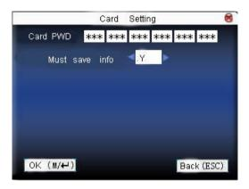
Press ▲/▼ to move cursor to the item to be set. If it is the input box, press numeric keys on small keyboard to input the value. If it is the roll box, press ◄/► to switch the values. After setting, press menu directly to return to the last interface. Press "ESC" to cancel setting and return to the last interface.
