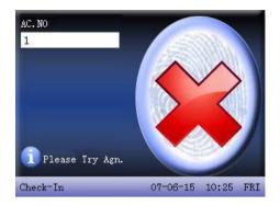
Employee can try another 2 times by default. The repeated times can be set in 4.5 interface option. If it fails after 2 times, return Step 1 for second operation.
