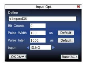
Input the name of user-defined format. Press  $\blacktriangle/\blacktriangledown$  to move cursor to the item to be set. If it is the input box, press numeric keys on small keyboard to input the value. If it is the roll box, press  $\blacktriangledown$  to switch the values. After setting, press **menu** directly to return to the last interface. Press "**ESC**" to cancel setting and return to the last interface.
