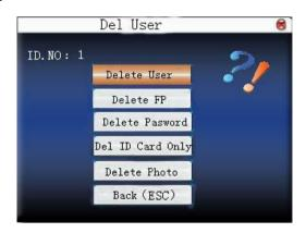
If the user has no fingerprint or password, the corresponding item is blue and cannot be operated. Press  $\triangle/\nabla$  to select the item to be operated. Press **OK** to pop out dialog box and verify whether to delete this item or not. Then the device will give corresponding prompt.
