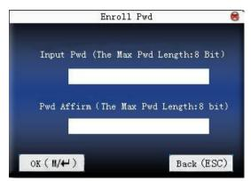
Input password (1 $\sim$ 8) according to device's prompt, and press  $\mathbf{OK}$  to verify it. Then press  $\mathbf{OK}$  save it or press  $\mathbf{ESC}$  to exit without saving it
