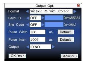
Input the name of user-defined format. Press ▲/▼ to move cursor to the item to be set. If it is the input box, press numeric keys on small keyboard to input the value. If it is the roll box, press ♣ to switch the values. For example, to modify failed ID as 10,press ♣ firstly to select "Yes", then input 10 in the input box.. After setting, press menu directly to return to the last interface. Press "ESC" to cancel setting and return to the last interface.
