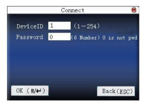
Press  $\blacktriangle/\blacktriangledown$  to move cursor to the input box. Press numeric key on small keyboard to input the value. After setting, press **menu** directly to return to the last interface. Press "**ESC**" to cancel setting and return to the last interface.
