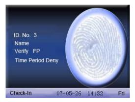
This means the current time is not in the time zone when employee is able to open the door. Therefore, the employee cannot open the door.
