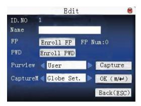
Work code cannot be modified. The operation is similar to that of **add user**. Fingerprint can be re-enrolled. Click "enroll password" directly to set password or modify password. The access can also be modified.
