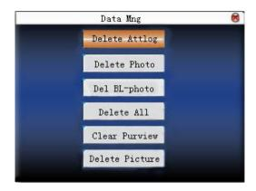
Press ▲/▼ to move cursor to the selected button. Press **OK** or **menu** to start operation. The device will remind you whether to continue the current operation or not. Then press **OK** or **menu** to delete all the data, which won't be recovered after deletion. Press "**ESC**" to return to the last interface.
