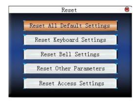
Press  $\blacktriangle/\blacktriangledown$  to move cursor to the button to be operated. Press **OK** to start operation. The device will say "Are you sure to execute the current operation?". Press **OK** to reset it to factory state and press "**ESC**" to cancel operation.
