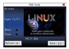
Insert U disk into USB slot of fingerprint sensor. Press " $\blacktriangle/\blacktriangledown$ " to preview the pictures in U disk. To upload the picture, click **OK**. Then the next picture will appear automatically. After upload, press "**ESC**" to exit.
