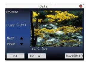
Press " $\blacktriangle/\blacktriangledown$ " to preview the propaganda pictures in the device. Click **OK** to delete all these pictures. After deletion, the next picture will appear. Click "**delete all**" to delete all the propaganda pictures in the device. Then press "**ESC**" to return to **data management** interface.
