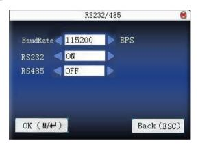
Press  $\blacktriangle/\blacktriangledown$  to move cursor to the item to be set. Press  $\blacktriangledown/\blacktriangleright$  to switch the values. After setting, press **menu** directly to return to the last interface. Press "**ESC**" to cancel setting and return to the last interface.
