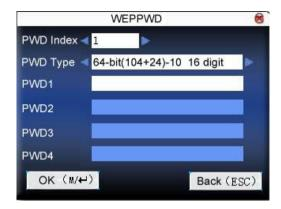
Input correct password. There are four passwords in **WEP password**. If the four passwords are set properly, only the current selected password is the effective value.
