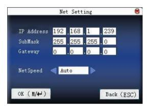
Press ▲/▼ to move cursor to the item to be set. If it is the input box, press numeric keys on small keyboard to input the value. If it is the roll box, press ◄/► to switch the values. After setting, press menu directly to return to the last interface. Press "ESC" to cancel setting and return to the last interface.
