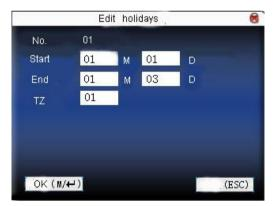
Press  $\blacktriangle/\blacktriangledown$  to move cursor to the input box. Press numeric key on small keyboard to input the value. After setting, press **menu** to save it. Then press **ESC** to exit.
