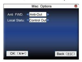
Press  $\blacktriangle/\blacktriangledown$  to switch the input box. Press  $\blacktriangleleft/\blacktriangleright$  to modify setting. Then press **menu** to save it. Press "**ESC**" to exit.
