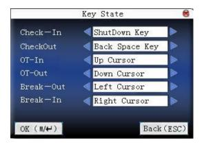
Press  $\blacktriangle/\blacktriangledown$  to move cursor to the input box. Press  $\checkmark/\blacktriangleright$  to switch the values. After setting, press **OK** save the setting. And press "**ESC**" to cancel setting and return to the last interface.
