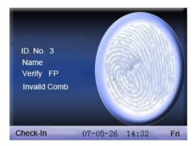
This means the group where employee is is not in the unlock combination. Therefore, the employee cannot open the door.
