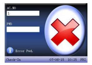
Employee can try another 2 times by default. The repeated times can be set in 4.5 interface option. If it fails after 2 times, return Step 1 for second operation.
