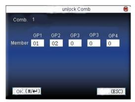
Press  $\blacktriangle/\blacktriangledown$  to move cursor to the input box. Press numeric key on small keyboard to input value. After setting, press **menu** to save it. Then press **ESC** to exit.
