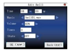
Press ▲/▼ to move cursor to the input box. Press numeric key on small keyboard to input the value. After setting, press **menu** directly to save the setting and return to the last interface. Press "**ESC**" to exit.
