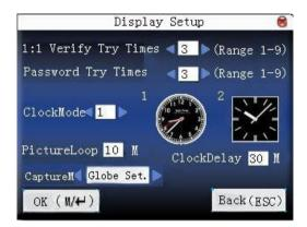
Press  $\blacktriangle/\blacktriangledown$  to move cursor to the input box. Press numeric key on small keyboard to input the value. After setting, press **menu** directly to save the setting and return to the last interface. Press "**ESC**" to cancel setting and return to the last interface.
