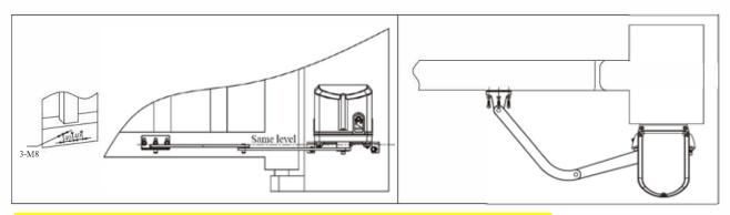
Notice: The front bracket and motor must be in same level!
